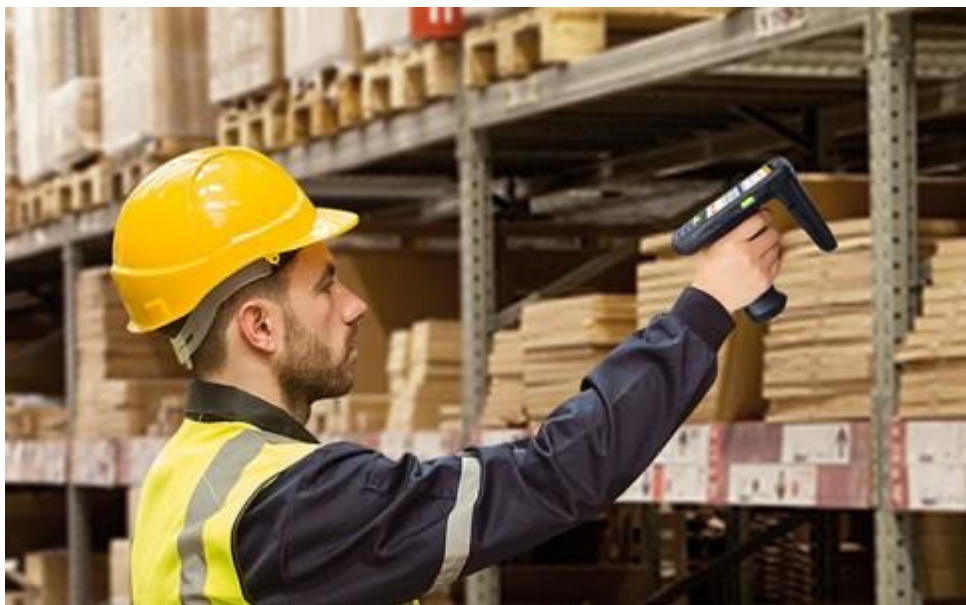
Slika 15: Komisioniranje uz pomoć RF terminala ( http://seuic.blogspot.com/2019/01/how-to-use-rf-handheld-scanner.html )
